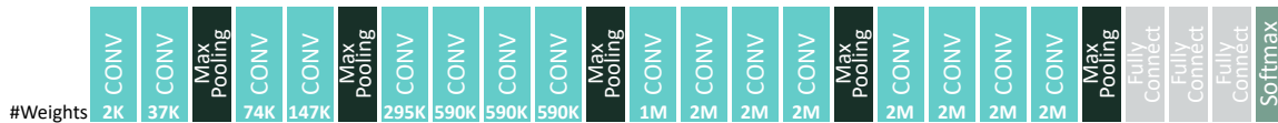
Fig. 2: VGG19 model architecture and the number of weights in each convolution layer.
